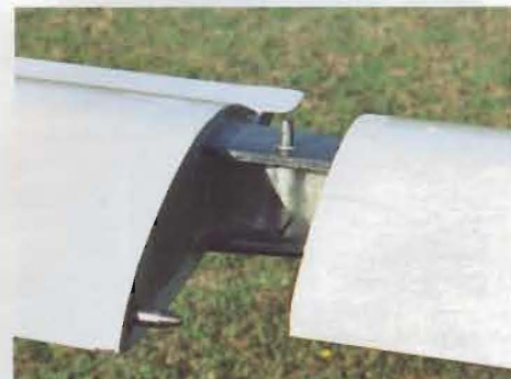
The Glasflügel 304cz's new 17.43m tips are fitted to the wing where the 15m tips would otherwise go
