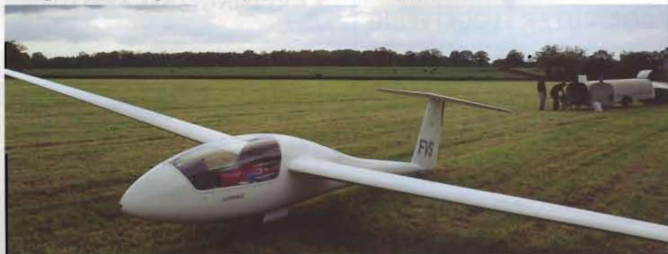
As some glider pilots have already found out, many vehicles are fitted with catalytic converters which, when parked heat up sufficiently to ignite stubble, straw or even dry grass. Take care when entering a field for a retrieve
